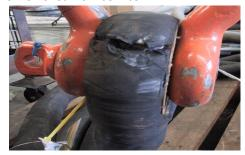
For heavy duty Kevlar® strops, the rear of the eye is well protected with many layers of rubberized heavy duty tyre cord. Depending on the severity of damage, the strop should be monitored, field repaired or removed from service.
