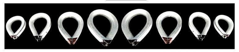
The 10t & 20t MBS Black Snake KEVLAR® range use embedded AS1138 wire rope thimbles. The low elongation properties of the KEVLAR® fibres do not deform wire rope thimbles at these low applied loads. The 30t and 50t MBS Black Snake KEVLAR® range only use AS1138 wire rope thimbles when the knuckles of larger shackles or oversize pins are required.
