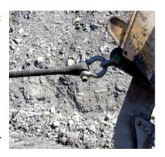
Lugs and pad eyes on the front of mining and road trucks must be linked to the vehicle chassis. Steel plate thickness and hole size should not allow undersize shackles to be mounted or installed. Bolster or cheek plates on lugs can be used to
