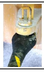
The cast clevis and pin arrangements on mining trucks must provide adequate strength and security when used with Body Up Safety Strops. These are safety devices. It is critical to calculate the maximum possible loads or seek OEM advice instead of assuming that all the equipment is properly matched. In the case of Body Up Safety Strops, failure of any component can lead to injury or death if the mining truck's dump body falls or is accidentally powered down to the chassis.
