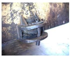
Maintain your recovery points in good condition and ensure they are strong enough. Black Snake engineered round eyes spread the load on pins to avoid high pressure point loading. Weld stronger recovery points on large vehicles by increasing pin/clevis size, use higher grade steel or consult with your equipment supplier for well engineered solutions. Remember that all steel work must be stronger than the recovery strop.
