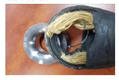
This damage is the result of doubling the strop around a shackle pin or similar. This strop cannot be repaired. Consider changing recovery procedure or strop length.
