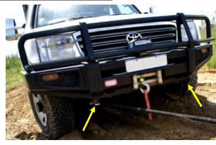
Well engineered light vehicle recovery points match our range of light duty nylon (8t MBS-12t MBS) strops. The photo (left) show an accredited aftermarket tow hitch in place of the towball mount. NEVER USE A TOWBALL! Aftermarket front mounted bullbars must have chassis mounted recovery points. NEVER USE VEHICLE SHIPPING LUGS OR LASHING POINTS!
