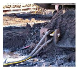
Skid mounted plant and specialized equipment will generally have pin/clevis or inbuilt heavy lugs (pad eyes) with plate thickness and holes designed for shackles of a certain size. Ensure that shackles are correctly matched to the recovery strop. Safety bow shackles (with bolt and nut) are preferable to screw pin shackles. Ensure that personnel are correctly trained to attach these shackles to equipment and strops.
