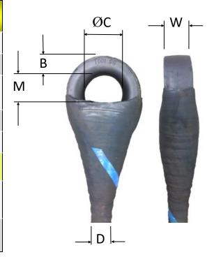
Custom designed and machined eyes are created from high strength, low alloy steel hollow bar. The bore hole is designed to minimize elongation under very high loads and to suit appropriately large shackles. We are always designing for safety and therefore undersized shackles (Jaw width) will not fit on the machined eyes. For example, a 17t S Grade shackle will not fit a 150t strop.
