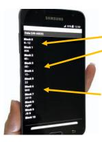
**Step 3:** Analyse embedded data Blocks 0 1 provide strop serial number Blocks 2 3 4 5 provide product code
